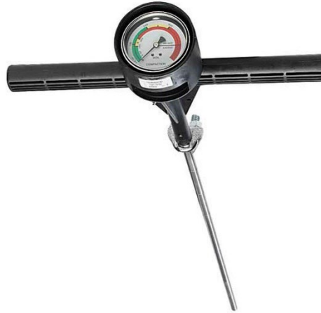
Figure 11. Cone scale penetrometer image
